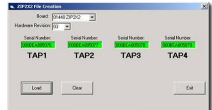
**Figure 2.** The JTAG software can match unique software to targeted boards and download common software code all in one test and programming cycle.
